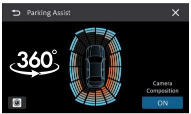
When reversing, parking assist guidelines appear on-screen, with an optional adapter for a 360-degree<sup>2</sup> camera view. <sup>2</sup> Subjected to vehicle model availability and suitability
